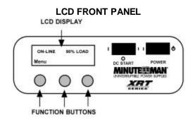
The XRT1000 through XRT2000 units have a 32 character LCD display, three push buttons, and the Pow er On and DC Start switches. (Both 120 and 220 VAC versions)
